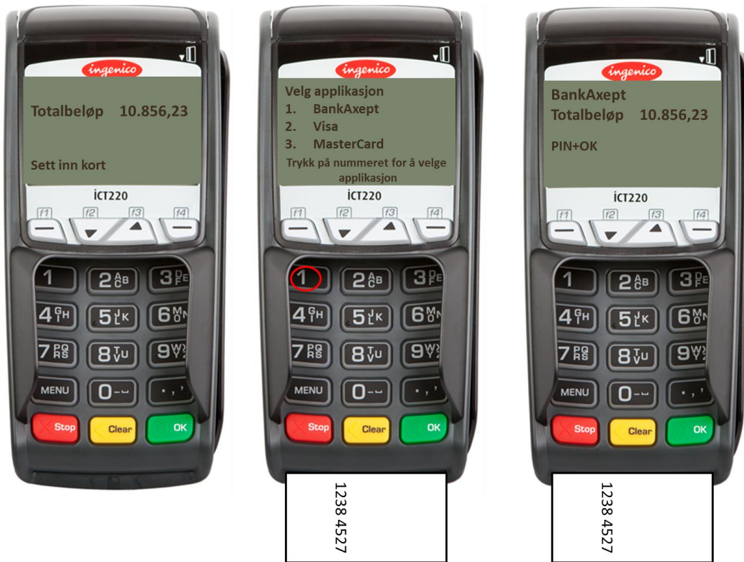
Figure 5: An override option using the upfront selection screen before the EMV payment process starts
