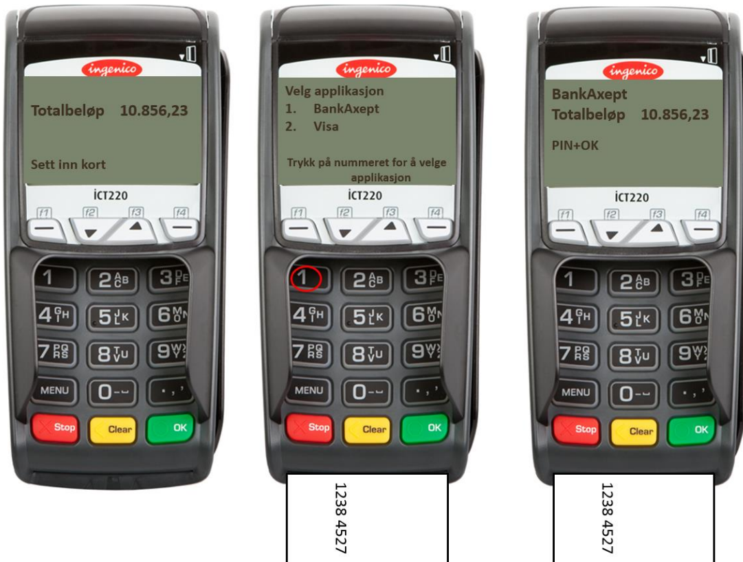
Figure 6: A choice of application by the sole cardholder during the EMV payment process
